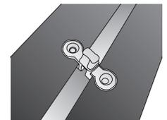
2. Line up the valance clips with the hooks on the blind. You can easily slide the hooks on the head rail to match the position of the hooks.
