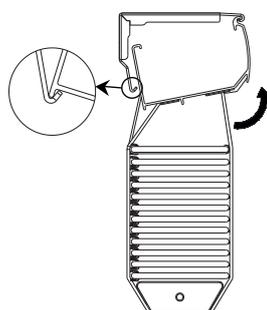
3. To remove headrail - push the headrail face to release from bracket and lower the front face (reverse of installation - step 1).
